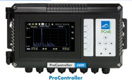
4-20 mA and digital inputs, e.g. data from external devices and plant stop signals Comprehensive in-built data acquisition, with full PC-ME DUST TOOLS software connectivity
