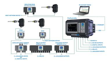
Figure 5: Typical multi-sensor layout
