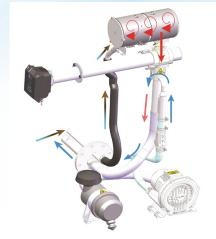
The QAL 182 WS utilises direct extractive heated sampling which can be configured to either extract an isokinetic sample or extract a sample based on a pre-set user-defined velocity. The extracted sample passes directly into a heated vaporising chamber. The sample is super-heated and exits into a controlled sample chamber. The *ProScatter*<sup>TM</sup> sensor provides a high accuracy, high resolution measurement meeting ELV's of 15mg/m<sup>3</sup> or less.
