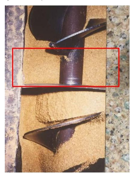
Remove section of screw conveyor so the ENVEA only measures the material
