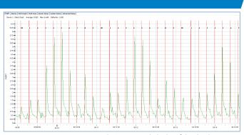
PC-ME DUST TOOLS 'Predict' – Line graph display of dust levels and bag-row identifiers during an on-line cleaning sequence
