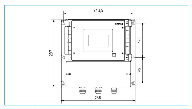
Fig. 8: Dimensions of the MSE 300 in the field housing (front view)
