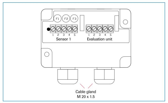
Fig. 14: Electrical connection of C1-Box
