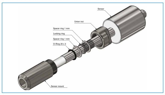
Fig. 6a: Installation of sensor in the sensor mounting
