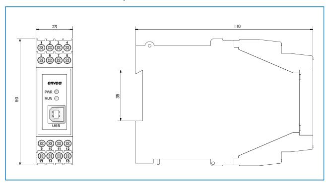
Fig. 7: Dimensions of the MSE 300 in the DIN Rail housing
