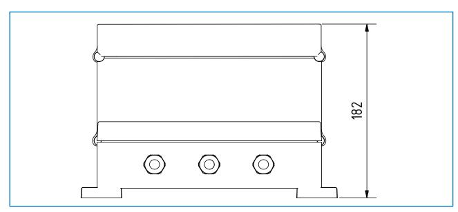
Fig. 9: Dimensions of the MSE 300 in the field housing (side view)
