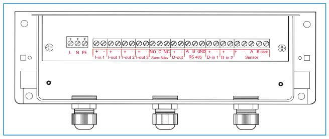
Fig. 13: Electrical connection of MSE 300-FH
