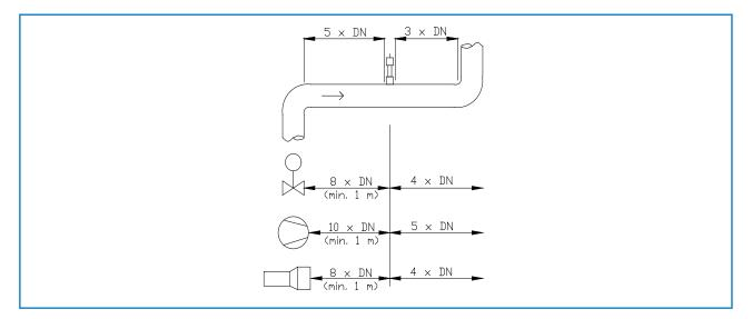
Fig. 4: Minimum distances of the measurement point from pipe geometries and fittings
