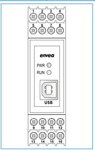
Fig. 12: Electrical connection of the MSE 300-DR
