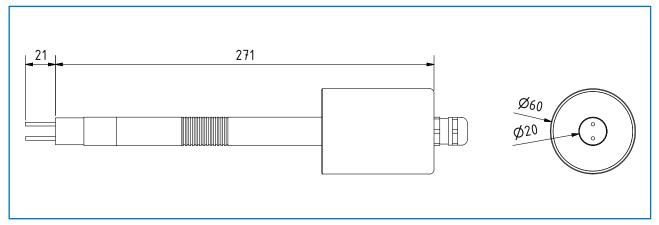
Fig. 11: Dimensions of the SpeedFlow 2.0 sensor
