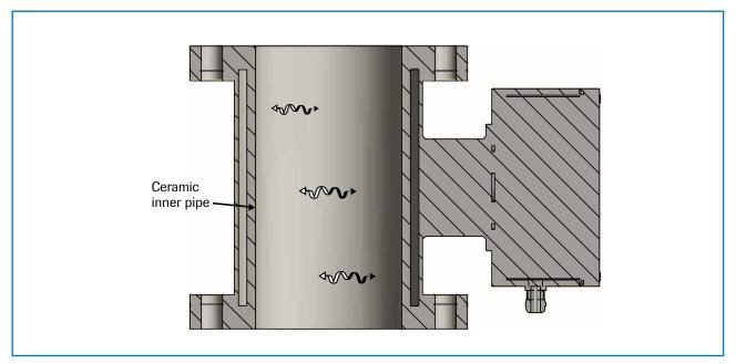
Fig. 3: Coupling of the electromagnetic waves
