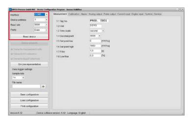
Select the correct COM port and connect to the device using the "read device" button.
