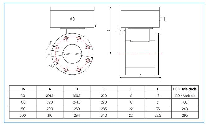
Fig. 5: Dimension of MaxxFlow HTC sensors
