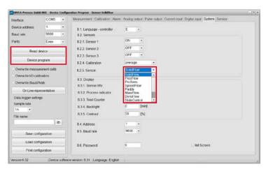
In the menu "System", under "Sensor" (8.2.5 or 7.2.5), the correct sensor must be selected.
