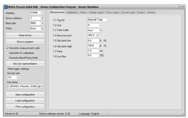
Communication is established by clicking on "Read device". The acknowledgement message "Parameter read in" is displayed. If an error message is displayed instead, check the communication parameters and cable connections between the PC and the transmitter.
