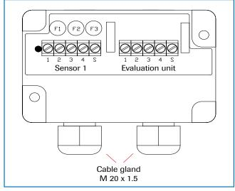
Fig. 13: Electrical connection C1-Box
