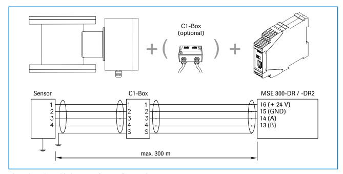
Fig. 2: Overview with C1-Box and DIN Rail transmitter
