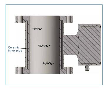
With the design in DN80 mm, the connection flange could be freely selected.
