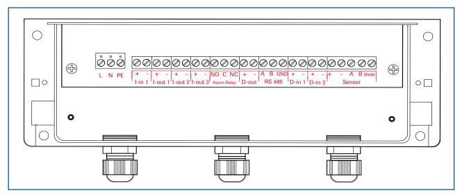
Fig. 19: Electrical connection
