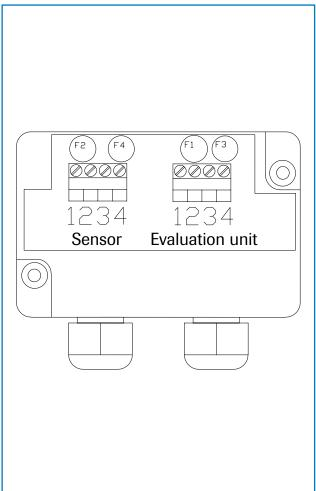
Fig. 17: Electrical connection of the Evaluation unit
