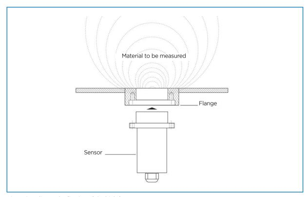
Fig. 5: Coupling and reflection of the high frequency
