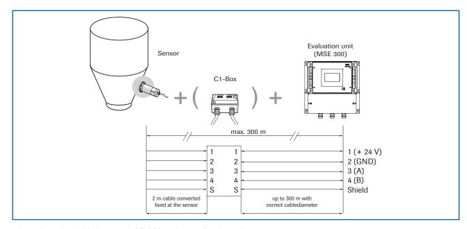
Fig. 2: Overview with C1-Box and field housing Evaluation unit
