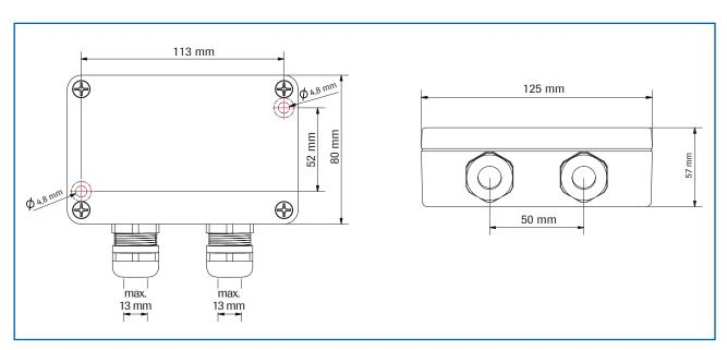
Fig. 14: Field housing for the C1-Box
