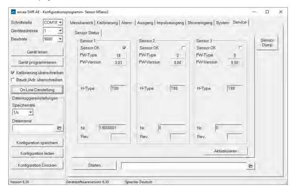
The status of each connected sensor is displayed in menu 8. Service. FW type, FW version, temperature, serial number and possible hardware errors are automatically read and displayed.
