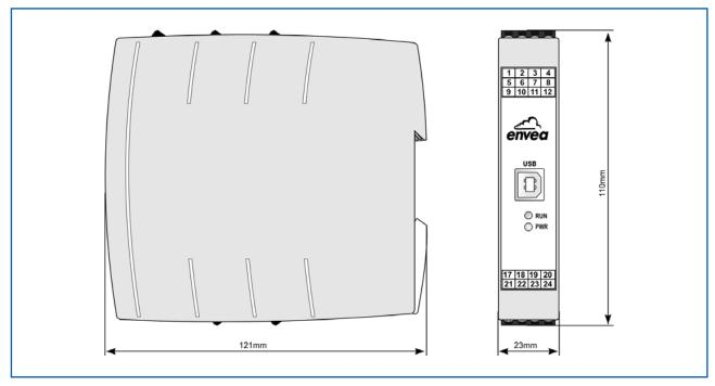
Fig. 12: Dimension of Evaluation unit in DIN Rail 2 housing
