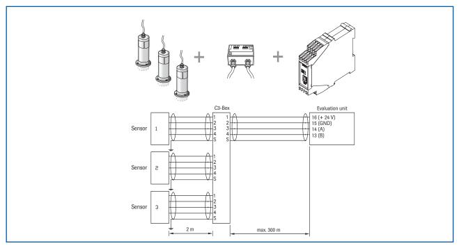
Fig. 4: Overview with C3-Box and DIN Rail Evaluation unit
