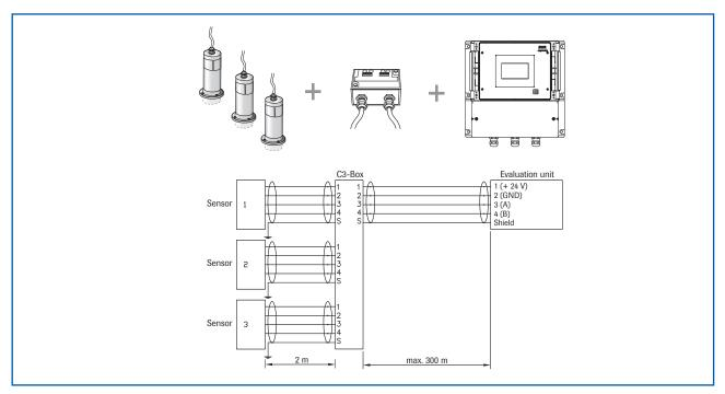
Fig. 3: Overview with C3-Box and field housing
