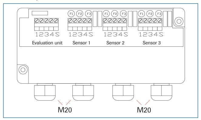
Fig. 20: Electrical connection for the C3-Box
