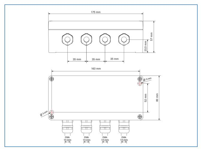
Fig. 15: Field housing for the C3-Box
