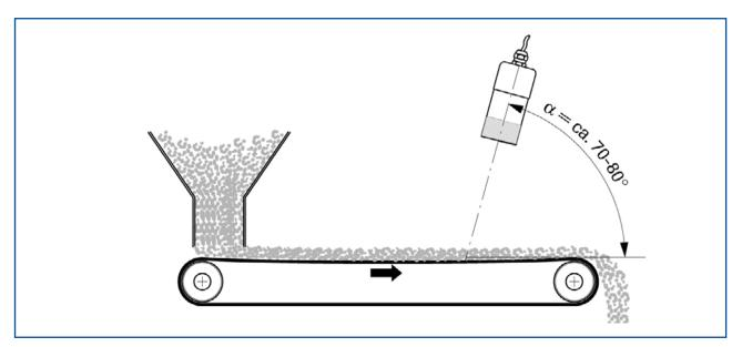
Fig. 7: Installation above conveyor belt
