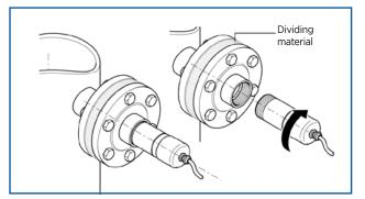
Fig. 6: mounting with separating flange
