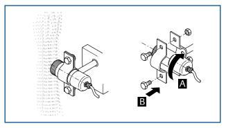
Fig. 5: Mounting with pipe clamp
