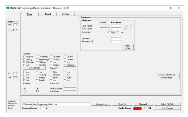
Upcoming errors are displayed here. A detailed error description takes place in the chapter Fault Clearance. The relay states are indicated by setting a hook on **Flow** or **Jam**.
