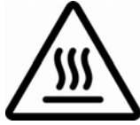
Temperature Hazard Caution or Warning
