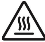
Temperature Hazard Caution or Warning
