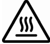
Temperature Hazard Caution or Warning
