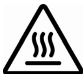
Temperature Hazard Caution or Warning
